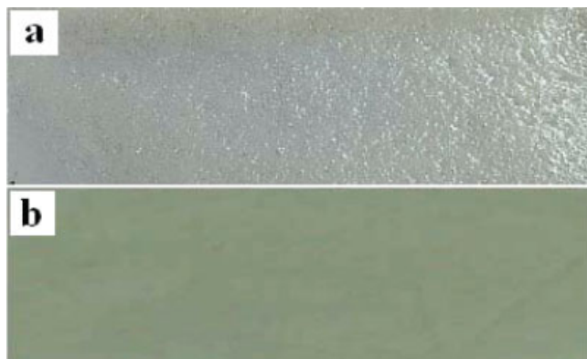
Figure 5 The photographs of the cured sheet of SPU with or without the synthesized 2-phenyl-3-hydroxyethyl-1,3-oxazolidine. (a) SPU/2-phenyl-3-hydroxyethyl-1,3-oxazolidine: 100/0, (b) SPU/2-phenyl-3-hydroxyethyl-1,3-oxazolidine: 100/10. [Color figure can be viewed in the online issue, which is available at www.interscience.wiley.com .]
